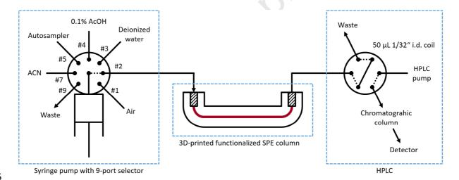
**Fig. 2**. Scheme of the flow setup integrating the 3D printed AuNP-decorated covalently immobilized monolithic structure as a front-end to HPLC separations.
