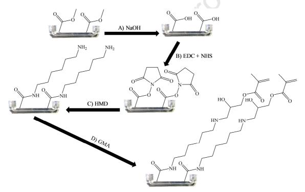
**Fig. 1.** Scheme of the sequential chemical modifications of the inner surface of acrylate-based 3D-prints prior to *in-situ* monolith preparation. The reagents used for the modification of the inner surface of the 3D printed support are: EDC: 1-Ethyl-3-(3-dimethylaminopropyl)carbodiimide; NHS: N-hydrosuccinimide; HMD: hexamethylenediamine and GMA: glycidyl methacrylate.
