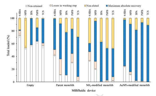
**Fig. 4.** Breakdown of the loaded mass of target analytes onto the different monolithic phases attached to the 3D-printed millifluidic devices for automatic SPE. The maximum absolute recovery was achieved for a total elution volume of 400  $\mu$ L with off-line detection. Error bars are given as SD values for three extractions performed with the same 3D-printed device.
