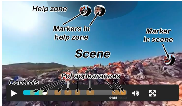
Figure 7: User interface of the interactive player, featuring the markers in the scene, the help zone with its markers and the controls with its PoI appearances.
